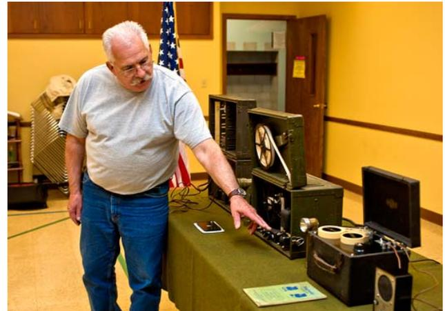
Yet another machine, much smaller than the first two, read a different kind of paper tape with short and long holes punched through it. A mechanical arm made contact through the holes and shorted terminals momentarily for the small holes and longer for the large holes! I had rigged up a little Code Oscillator with a light so the boys could see and hear the code being "read".
