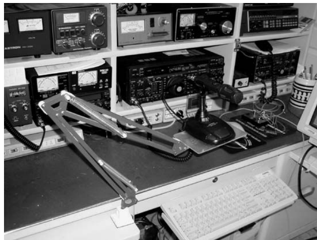
The converted articulated lamp arm holding the MD-100 microphone and stand.
