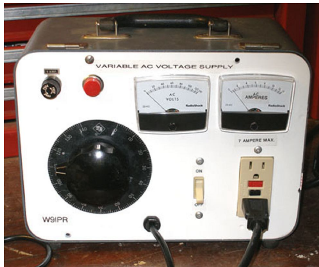
A variable AC Voltage Power Supply using "junk box" parts.
