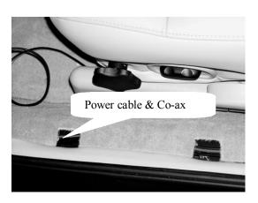
The molding was temporarily removed below the driver's seat to allow the wires to be fed forward and remain out of sight and protected by the replaced molding. These moldings are not screwed in but snap in and out.
