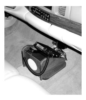
The wires were then secured to the underside of the dash using tie-wraps with adhesive pads and routed to the area of the transceiver. The original fuses were retained at the transceiver and the 30 amp Anderson power pole connectors were used to make the power connections. I prefer these as the common connectors since it allows the transceiver to be easily pulled from this car and used in the truck or as a base station both of which are also equipped with these "power pole" connectors.
