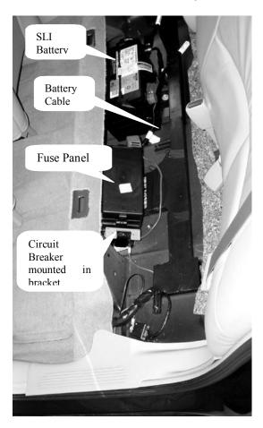
The #10 power cable from the circuit breaker and the RG-58 antenna co-ax were then slipped under the floor molding and fed in the direction of the driver's side door.
