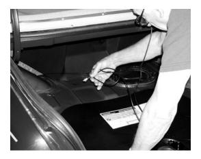
The RG-58 co-ax from the antenna was then passed through a wiring harness passage behind the rear seat.
