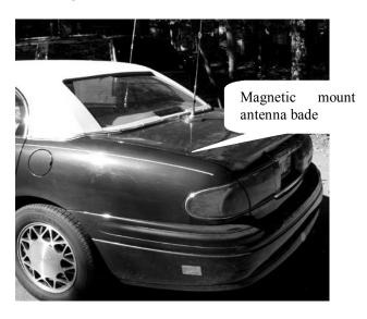
The Buick has a metal trunk lid so a dual band magnetic mount antenna was used. The co-ax from the antenna is small so it was laid along the trunk lid gasket to enter the trunk area. I have used this approach before without damage to the co-ax.
