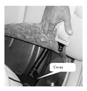
Since the cable passed along side a wiring harness there was no hole required in rear bulkhead.
