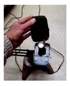
Now the converted battery unit is reinstalled in the drill and is ready for use as powered by an external 12 volt battery. Note the use of the Anderson Power Pole connectors
