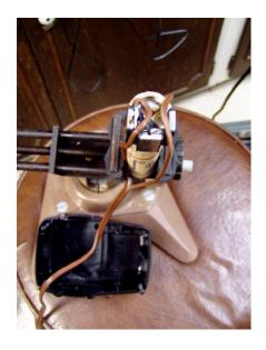
Now as the battery compartment is reassembled with the cord through the back of the case the secured case will hold the battery and contacts in place.
