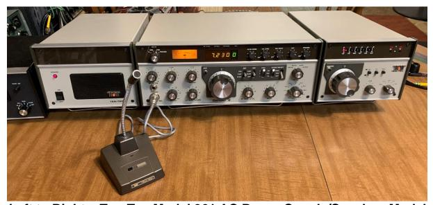
Left to Right – Ten-Tec Model 961 AC Power Supply/Speaker, Model 561 Corsair II Transceiver, and Model 263G Remote VFO.
