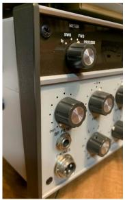
To the left you can see the assembled End Cap on the left side of the Corsair II Transceiver. Remember the tabs on the Ten-Tec End Cap in the above picture. Those Tabs slide behind the screws you can see at the top left corner and lower left corner of the Corsair Front Panel. Older Ten-Tec gear will often have one of both of those tabs broken off from misuse at some time in their past. As far as I know, Ten-Tec is the only source for these End Caps – and they no longer supply them.
