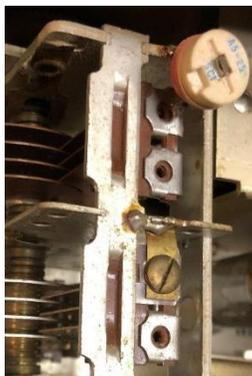
Notice in this closer view that the brass clip – that was the original compression trimmer – has been removed in the process of adding the new trimmer. The trimmer was supplied by Hallicrafters to customers.
