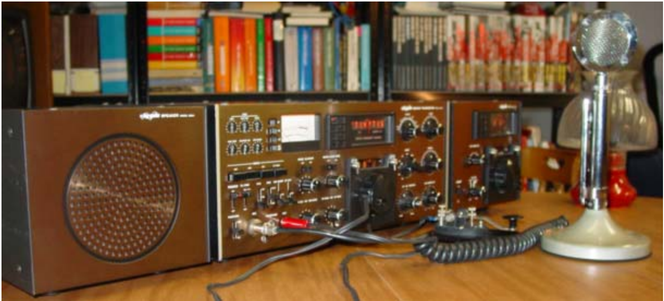
HyGain 3750 Complete Station in about 2010 Left to Right are the 3854 Speaker, 3750 Transceiver, and 3855 External VFO (Note also the Astatic D-104 Microphone and Nye-Viking Straight Key W9MXQ Photo
