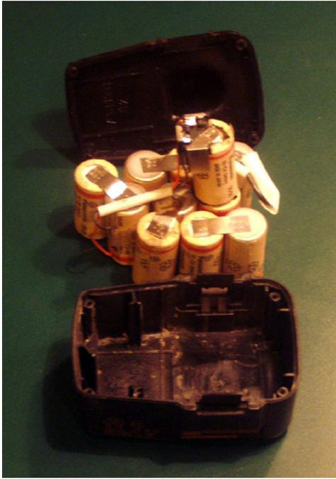
After a couple of hours I noted three cells in the string measured about 1.4 volts and could be reused while the other six were shorted, measured about zero volts and were not reusable.
