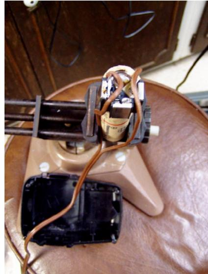
Now as the battery compartment is reassembled with the cord through the back of the case the secured case will hold the battery and contacts in place.
