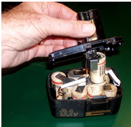
First I removed the four screws that held the battery case together and studied the battery configuration.
