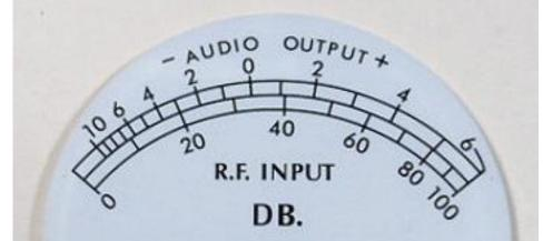
This is a Honeywell meter face kept as a spare at W9MXQ. Some 51S-1 Receivers are equipped with a Bartlett meter. Those meters have a slightly different appearance. The scales are the same, however.
