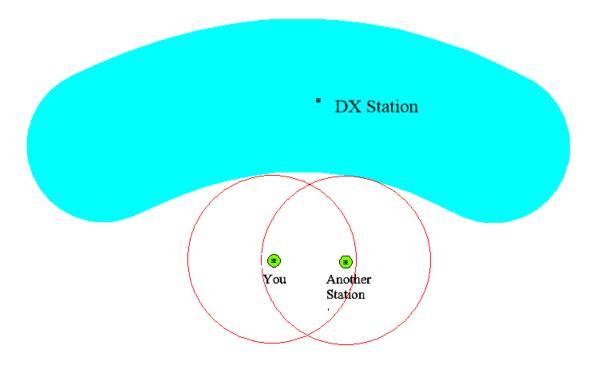
Skip zone example. The green areas represent the ground wave distance. The areas inside the red circles are the skip zone. Signals originating inside the skip zone and outside the groundwave area cannot be heard. Both of you can hear stations in the light blue area. The DX station hears both of you.
