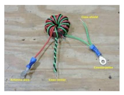
The transformer is placed in a box with an SO-239 and two bolts with wing nuts for attaching the antenna wire and an optional counterpoise.
