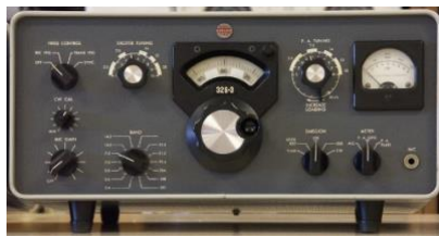
32S-3 Transmitter Standard Coverage (W9MXQShack Photo)
