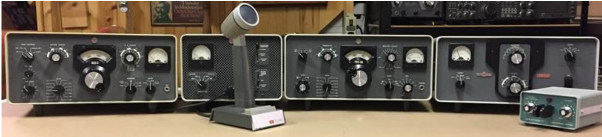
Collins 32S-3 Transmitter, 312B-4 Console, 75S-3B Receiver, 30L-1 Linear Amplifier Also, Shure 444 Microphone and Heathkit HD-1410 Keyer Initially, the amplifier was the floor mounted 30S-1 – the 30L-1 came slightly later (W9MXQ Shack Photo) (Not shown is the Collins 516F-2 AC Power Supply – installed out of this view)
