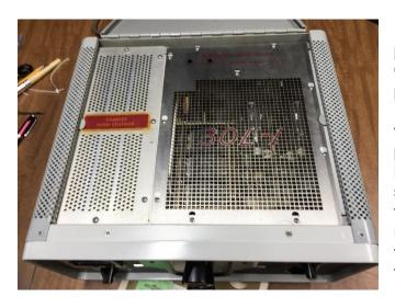
Here is a view of the 30L-1 Linear Amplifier with the cabinet cover door open. Compare this with the above interior picture and see both the Power Supply (left) and RF Compartment (right) covers in place. See also the unique punch pattern for the RF Cover that allows the model number to be silk screened in the active area of ventilation holes. The 30L-1 is an impressive mechanical design. That and the electrical design have withstood the test of time.
