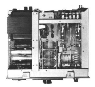
At the left here you can see in interior view of the Collins 30L-1 Linear Amplifier the Power Supply and separate RF Area shields removed. This picture, from the 30L-1 Technical Manual, does not show the more modern retro-fit power supply board installed at the lower left hand corner of the radios.
