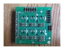
To the left is the Young Kim, K6HM, retro fit HV Circuit Board. The capacitors are on the understand of the board. The HV diodes are shown across the top and the top right, The equalizing resistors are on the left and under the capacitor rows. The Harbach board is equally well designed and of excellent quality.
