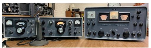
Collins KWM-2 and 312B-5 (1961) with a Hammarlund HQ-170AC-VHF Receiver (1958). Transmitting with the Collins and Receiving with the Hammarlund.
