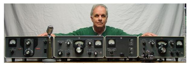
The W9MXQ Collins S-Line Station – Pictured from my QRZ Page 30L-1 Amplifier, 75S-3B Receiver, 312B-4 Console, 32S-3 Transmitter W9MXQ Collection
