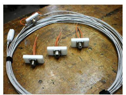
The finished product is shown at the left. If I only have one coaxial line available, I can easily switch between antennas. If there are other operators who have a cable but no antenna, they can also make use of an uncommitted one.
