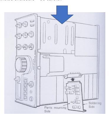
Once the daughter board being serviced is removed, the radio is turned on its side, as shown, and the board's connector is unscrewed form one side and hinged outward, away from the chassis. The removed daughter board is then re-inserted into the connector to allow it to operate while being accessible. The arrow points to the only area of boards that cannot be serviced in the way described herein.
