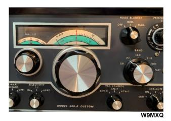
The Frequency Determination Controls on the Swan 600-R Custom Receiver – Typical if the 600-T, 600-R Standard, and the 600-R Custom.
