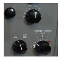
Earlier, the Sideband Selection and Mode switching in the HQ-170 was described. That also is similar in the HQ-180 and HQ-180A Receivers. However, the control layout is different. The VERNIER TUNING control for the HQ-180 series radios is to the right of the right main tuning window and is a smaller knob than on the HQ-170 series. The VERNIER TUNING knob location on the HQ-170 is the BFO KCS.
