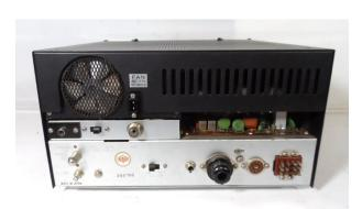
In this rear panel view, note the exposed internal circuitry at the right center – an open area to the interior. While probably not a shock hazard at that location<sup>4</sup>, it left circuitry exposed in an otherwise well enclosed cabinet design. Connections below the fan were for an external receiver. See connections for the PS-511S Power Supply and VFO-5SS Remove VFO. To the right of the fan is a connector that is used to get fan power from the PS-511S Power Supply.
