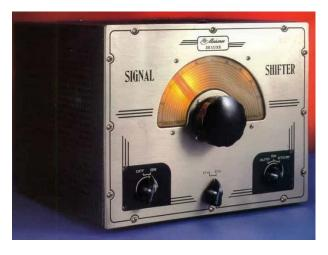
This picture is typical of the Variation 2 product under models 9-1077, 9-1078, and 9-1080. These dated from 1943 and through World War II. This little Transmitter/Exciter produced 7.5 watts output using ham band and general coverage (HF) RF coils. It was intended to run alone or with the 150-B Amplifier that had a complete audio circuit and modulator. Although low in power, the Signal Shifter could operate barefoot.
