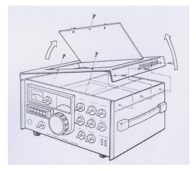
Here is a picture of the opening of the cabinet. Screws are removed from the top and right side, as shown, to allow the complete cabinet top to open via left side hinges to expose the entire top of the radio.
