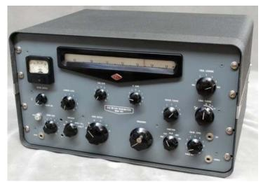
Gonset GSB-100 HF (80-10 Meters) SSB/AM/PM/CW Transmitter<sup>4</sup>
