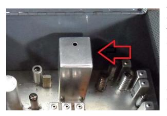
This large assembly in the back center of the radio chassis – reference the red arrow – is absent from HQ-170 and HQ-170A Receivers. It is present only in the HQ-170AC-VHF. Contained therein is a converter and pre-amplifier for 2-meters. The converter and pre-amplifier use the then new, and revolutionary, Nuvistor vacuum tube from RCA. Not much larger than a transistor, it was designed with its tiny internal elements to be effective at VHF and UHF frequencies.
