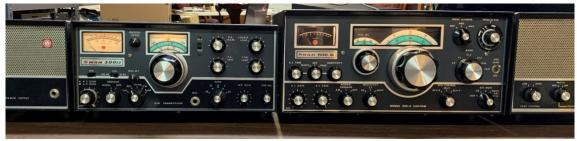
Swan 500cx Transceiver with Swan 600-R Custom Receiver (with 117XC Power Supply/Speaker and 600-SP Speaker/Phone Patch)
