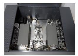
Non- "A" Series HQ-180C See the 5U4 Rectifier at the left rear, the heat generator! W9MXQ
