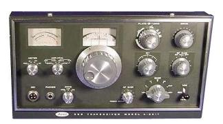
Allied Radio A-2517 HF Transceiver from 1970. This perhaps is the first Trio-Kenwood radio to be marketed in the USA. Comparing this radio with the Trio TS-510 shows them to be similar, if not identical. There was also a very nice A-2516 Receiver that would have worked well as a partner with the A-2517 shown here. The A-2515 was not designed to transceive with the A-2517, to my knowledge. These date from about 1970.
