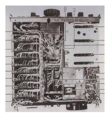
This is the TS-900 Bottom View with the front panel at the top of the picture. You can see the wiring harness "motherboard" that allows for the hinging of the PC board sockets for the Daughter Boards to be hinged outward for access while in operation. The boards available for this process are along the left side of this picture, at the bottom half of the center area. However, the i-f related boards at the picture's upper right (with the shield covering them) cannot be serviced in this way.
