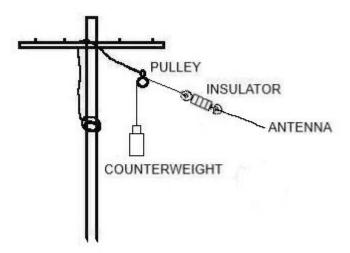
The counterweight keeps the antenna taut so there is very little "belly", and high winds, ice or snow offer no danger to the antenna's position. But, as we have seen, a falling tree will bring it down (without breaking it), until it pops back up when the tree is removed.
