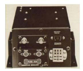
Kenwood DS-900 12VDC Input Power Supply. The large Jones Connector is for connection to the TS-900 Transceiver. See the AC Socket at the upper right-hand corner. In this picture that is shown as 220 VAC – presumably because this picture is for a European version. That outlet would have been 120 VAC in North America – presumably to power the VFO-900 Remote VFO that contained its own internal AC Power Supply (but provided for 12 VDC operation).
