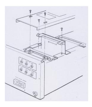
Here is a picture of the removal of top shields (covering the installed daughter boards) for individual board access. Note that each board is held in place with two screws.
