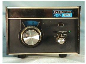
The Drake RV5 External VFO was never produced, as noted in the text. However, it was identical to the RV7 except for tuning direction. I am reasonably sure that this prototype unit was made from pieces of an RV7.
