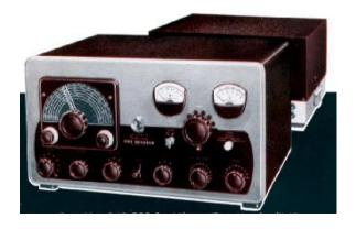
The Johnson Viking 500 was a massive, 173-pound radio in two cabinets. The desktop unit held all the RF components and control circuitry while the second unit (intended to sit on the floor) contained the power supply and modulator components. This unit provided 500 watts input of plate modulated AM Phone and 600 watts input on CW.
