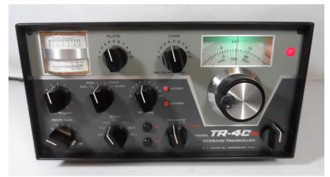
Drake TR-4CW/RIT HF (80-10 Meters) SSB/AM/CW Transceiver
