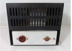
At the left, top picture, is a front panel view of the VFO-5SS Remote VFO. The VFO takes its power from the host TS-511S transceiver. Note there is a crystal socket at the upper right-hand corner and an associated crystal/VFO switch below it. The VFO-5SS could use a crystal for a single frequency location, such as a net. This was much more important in a day when free running VFO oscillators could not approach crystal stability like the PLL circuits of today.
