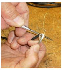
moved; poke around and gently separate the braiding. Then put the tool between the center conductor and the braiding, push through, and slide the center conductor out.
