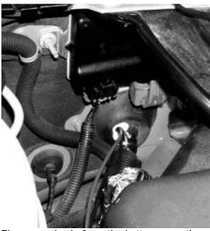
The power leads from the battery were threaded along a main wiring harness that already passed through the firewall using a blunted clothes hanger. I was especially careful to avoid damage to any of the existing wires in the factory harness.
