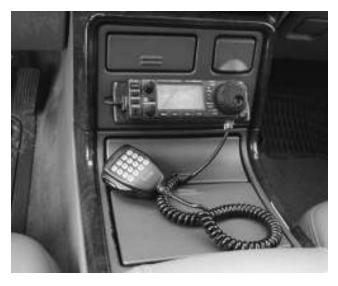
The completed control head installation provided a dash mount with rear wiring access and most importantly, wife approval. Plus, it's easy to see and operate.
