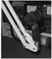
The adapted mic holder is shown secured in the extension arm clamp.
