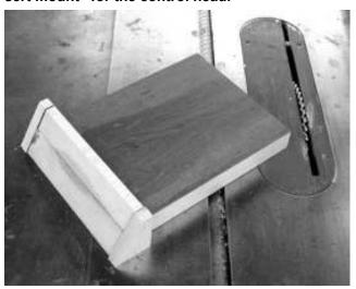
Using the table saw and some scrap lumber an insert was fabricated that would allow for the control head to be mounted on its sloping face.
