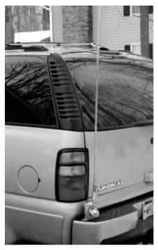
The HF antenna coax was also passed through the hatch door seal gasket and under the carpeting to the transceiver. Notice that the Hustler antenna was stabilized to the luggage rack using a stiff plastic rod (electric fence pole) and tie wraps.
