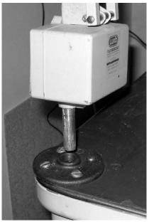
A  $\frac{1}{2}$ " pipe nipple and floor flange is used to assemble a secure desk swivel mount for the "mic econo-arm"
