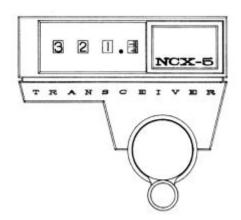
and shared pretty much by just National and Hallicrafters in those days. The most unique feature of the two was digital frequency readout. National did that with a mechanical (counter) mechanism as shown below:
