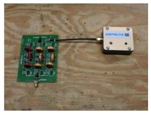
The device is called the WSPRlite (<a href="http://www.sotabeams.co.uk/wsprlite">http://www.sotabeams.co.uk/wsprlite</a>). It's a 200 mW WSPR transmitter that supports the 20m and 30m bands, and with the added Low Pass Filter kit it can operate on the 40m, 80m, and 160m bands. The WSPRlite transmitter comes assembled in a 2"x2"x0.75" enclosure. The only interfaces are a micro USB port for power and configuration, an SMA connector for an antenna, and a button to start transmitting.
