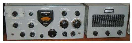
The KWM-1 Transceiver and the 312B-2 Speaker (the 312B-2 included a Speaker, Wattmeter, and Phone Patch)
