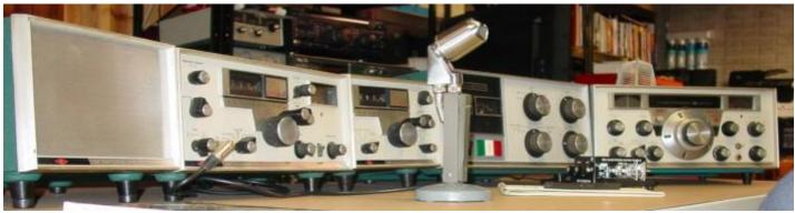
Left to Right are the National NCX-A AC Power Supply/Speaker, the NCX-5 HF Transceiver, the VX-501 External VFO, the NCL-2000 Linear Amplifier, and the HRO-500 Receiver. The HRO-500 here is acting as a second receiver with the NCX-5, when desired.
