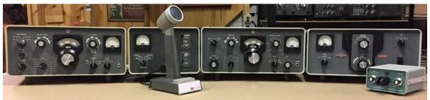
Collins 32S-3 Transmitter, 312B-4 Console, 75S-3B Receiver, 30L-1 Linear Amplifier Also, Shure 444 Microphone and Heathkit HD-1410 Keyer
