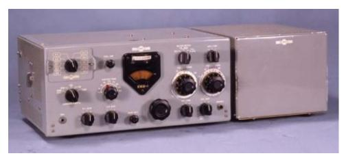
The KWM-1 Transceiver and the 516F-1 AC Power Supply
