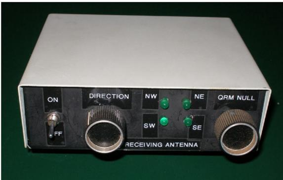
The control labeling was made using white lettering on clear tape in a labeling machine.
