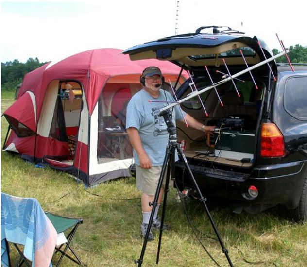
**Gary Bargholz (N9UUR) made his contact via the satellite using his FT847 transceiver and portable Arrow antenna**
