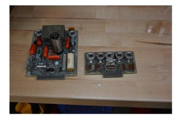
The above circuit boards from the HP 410C were replaced with solid state items, made by Kiss-electronics of Cornelius, Oregon, they were a two-minute job to install.
