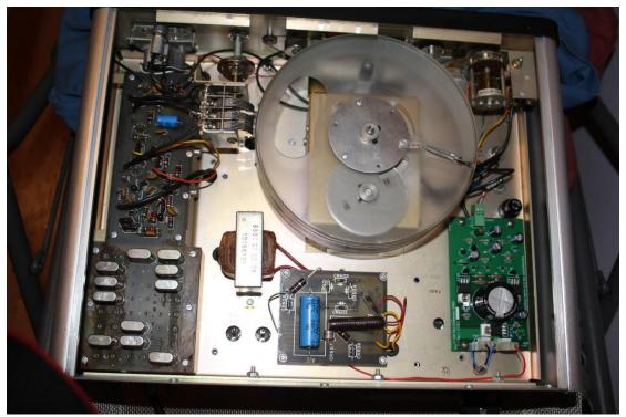
Bottom View – Hammarlund HQ-215 at W9MXQ – Front Panel at Top. Note two missing audio transformers at the lower right where the new W9AC Audio Amplifier is mounted. Also note the relocated
