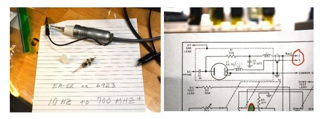
Only a few components were replaced in both the 1600 and 1600B Hickok meters, one selenium rectifier and three electrolytic capacitors. I left the old can type electrolytics disconnected in the chassis, just to allow it to look complete.
