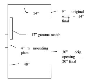
My original dimension was a total length of 114" and I fabricated a gamma match of 3/8" tubing 17" long with a 14" piece of RG-8 coax (less the shield) inserted inside the tubing as the feed capacitor. Initially I attempted to tune the antenna length and gamma match using my MFJ "259" antenna analyzer while in the garage. Big
