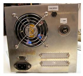
The fan, fan speed knob, fuse and the filtered AC input connector are all seen here.
