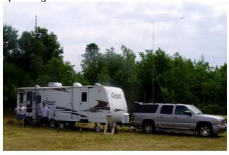
The 40 meter phone station was perhaps the most easily set up with simply the positioning of the travel trailer. Ed Frac (AA9WW) and Jake (KB9ZOR) are shown with the portable tower Ed got at Dayton and which supports the center of a dipole. The 40 meter "kick ass" vertical is shown in the distance behind the tow vehicle.
