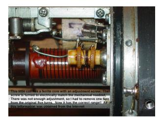
At the end of the electrical repairs, a complete RF and IF alignment was done. All tubes had been checked on my Hickok 752 and all were at 100%. The radio worked in a beautiful manner. The CW filter went down to 100Hz and it really worked well. The BFO started acting up, and would simply stop running. Upon some trouble shoot, I found bad resistors in both the plate a
