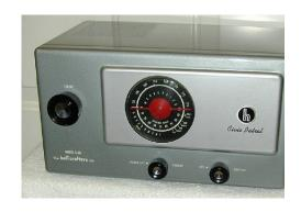
The previous owner was obviously a smoker. The interior was covered in that familiar brownish grime. The dial cord was broken and none of the tubes checked anywhere near "good". All four sections of the filter cap were bad and, of course, the pots were dirty and noisy.
