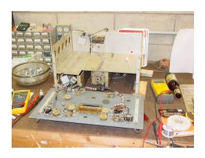
Please note the empty "fuel" container on the right side of this picture. The capacitors were all replaced, and several out of spec resistors. Then the RF deck gear train was 100% disassembled and all of the 46 year old grease removed one gear at a time. The gear train was re-assembled and aligned, a project that you do not want to do every night of the week. It is very demanding and requires perfection, for a proper function receiver.
