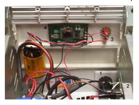
At 1 is the variable resistor for adjusting voltage. The bridge rectifier, bolted to the side panel, is at 2. The on/off switch for the battery is at 3, while the digital meter is at 4. An old pill bottle (thanks, Dave!) has been cut down to hold the battery at 5.
