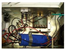
Above is a view looking down into the case. The junk box transformer is at 1, a heavy job with dual 10- and 12-volt taps, only one of which is used. The 12-volt tap supplies 17 volts
