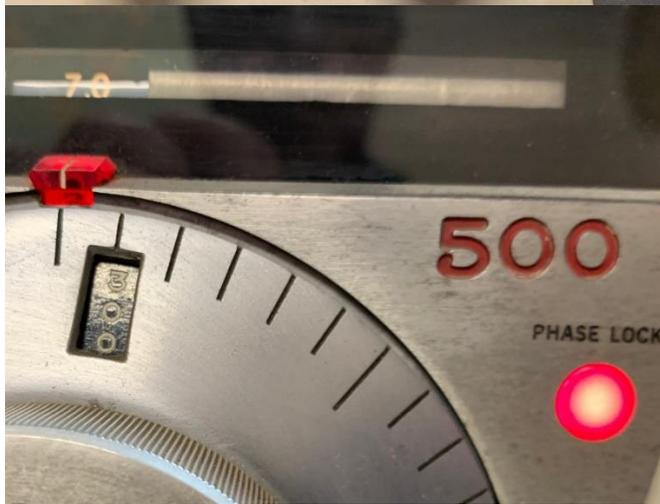
Reference above picture. Tune the SYNTHESIZER TUNE control until the readout over the main tuning dial says "7.0," meaning that the lowest frequency on the range we are tuning is 7.0 MC (MHz). Adjust the SYNTHESIZER TUNE control until the PHASE LOCK light (see at left) is extinguished. The SYNTHESIZER TUNE is now correctly set.
