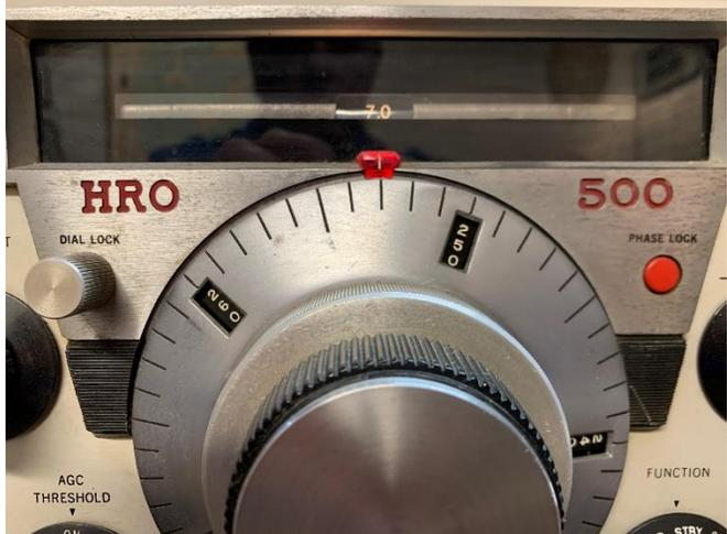
Using the readout window in the upper left-hand corner of the picture above, peak noise in the receiver speaker for maximum by adjusting the PRESELECT TUNE control. There is an arc in this readout window corresponding to each of the five frequency bands selectable with the BAND MC switch.
