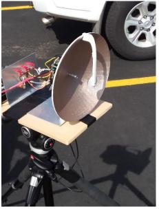
WF0T's 122 GHz rig. The dish is 3-D printed.
