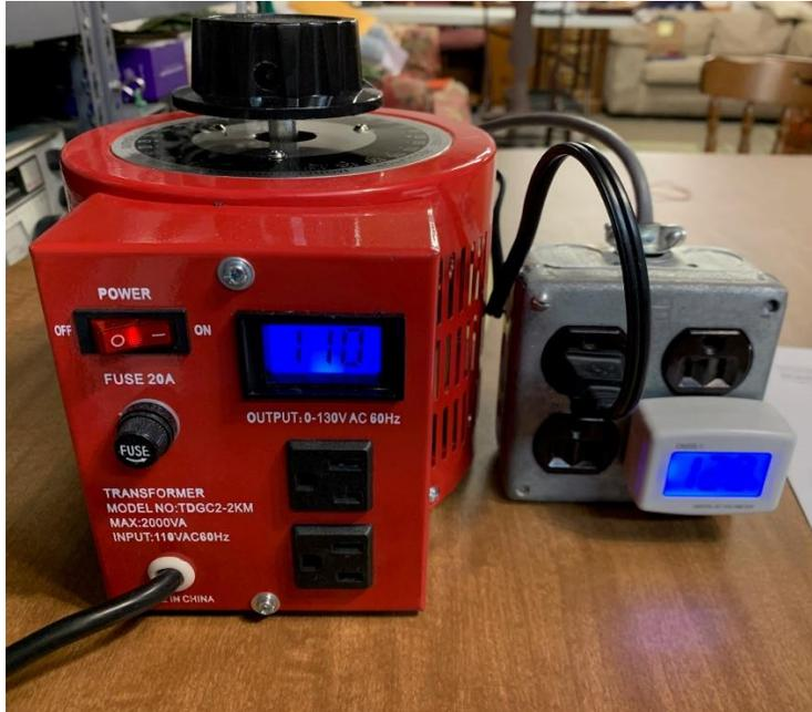
Meter on the autotransformer ("Variac™) is reading voltage to the radio or device/load connected. Hard to read here but it is 110 VAC.
