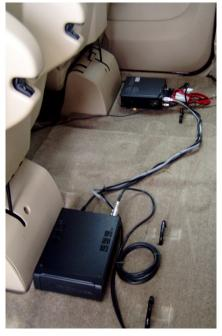
The previous vehicle had a bench rear seat with plenty of room for the transceiver and antenna tuner however in this vehicle, with separate "captain's" seats in the rear the units had to be located separately . A floor mat will cover the interconnecting cables.
