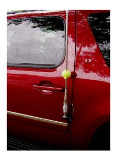
Temporally the HF antenna was mounted to a rear side door using a "lip mount". While this arrangement works OK and allowed me to check into the FL-Milwaukee net on 14.290 it just does not seem very secure and I will be replacing the mount with a type of hitch mount.
