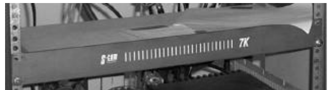
The controller routes audio from the receiver to the transmitter for rebroadcast and adds the station identification.
