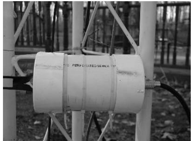
A ten-turn balun wound inside a length of PVC drainpipe.
