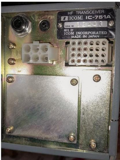
**Icom IC-751A without the Optional IC-PS35 AC Power Supply Fitted**
