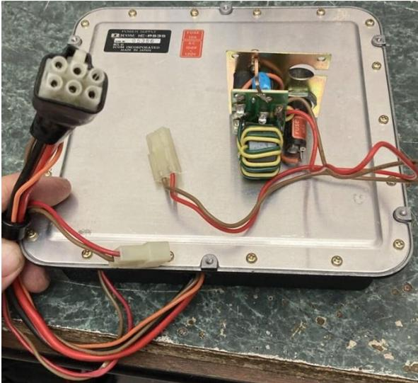
**Mounting Side of IC-PS35 AC Power Supply with Access Panel to the right and standard power plug to the left.**
