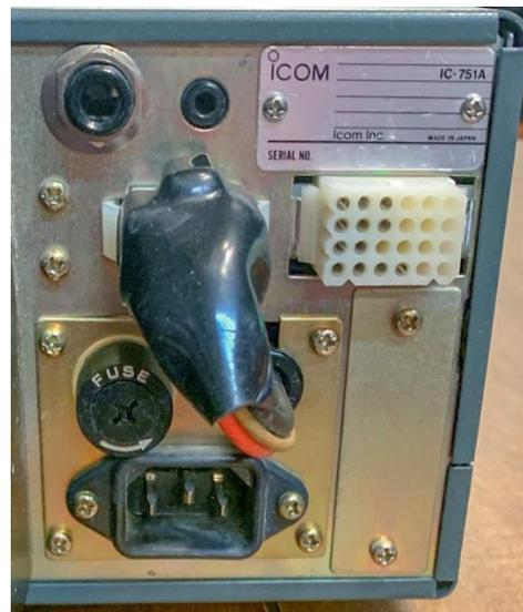
**Icom IC-751A with the Optional IC-PS35 AC Power Supply Fitted**
